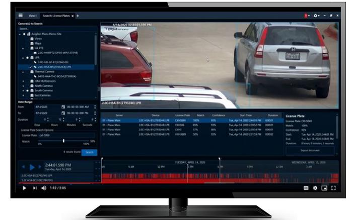
LPR analytics automatically read license plate information from vehicles, linking it to live and recorded video. This enables security operators to detect the presence of vehicles of interest in real-time or search, using full or partial numbers, and quickly find specific captured license plate video for further verification and investigation.
